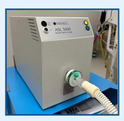
The ASL 5000 is a breathing simulator that allows for high-fidelity ventilation practice, designed to be used with almost any ventilator. At VGH SIM, the ASL 5000 can be used in combination with the SimMan Essential or one of our SimMan ALS.
