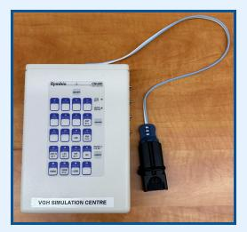
The rhythm generator allows you to simulate rhythms on a defibrillator without the use of a connected manikin/ShockLink device. This can be helpful for simulations that do not require high manikin fidelity.
